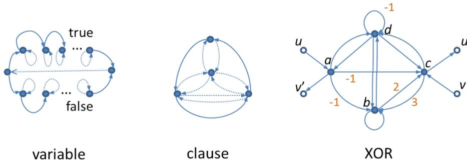
**Figure 1: Gadgets used in proving Valiant’s lower bound.** All edges have weight 1 unless noted otherwise. For the variable and clause gadgets, the solid (not dotted) edges are called (*vertex*) *external edges* or (*clause*) *external edges*. Note that the number of external edges in a variable gadget is not fixed, and need not be the same for the True and False halves of the gadget.
