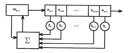
Figure 1: Feedback with Carry Shift Register
